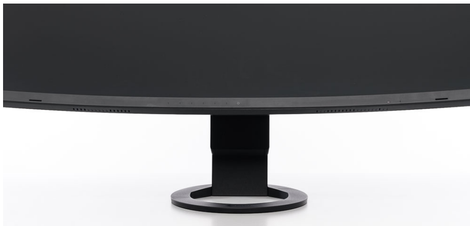
Front-facing speakers: Slots on the outer edges
