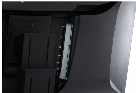
Connections on the right: Signal inputs
