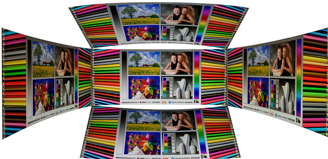
Horizontal and vertical viewing angles
