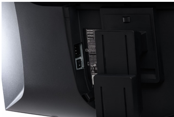
Connections on the left: Power and mains switch
